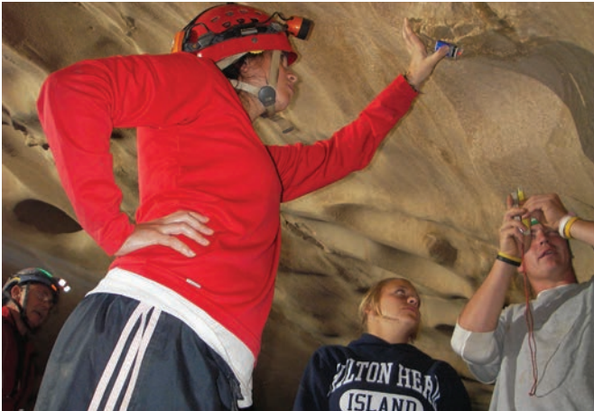
Clinometer short shot, Cascade Cave, Carter Co., KY. (photo by Horton Hobbs III)
