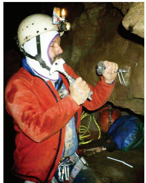
Setting bolts, Sinks of the Run Cave, Greenbrier Co., WV. (photo by Horton Hobbs III)
