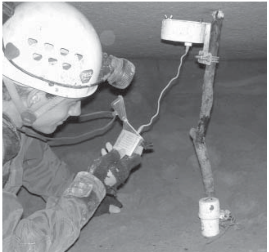
Figure 4. Downloading humidity and temperature data.
