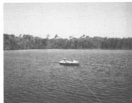
Rainbow Blue Hole. The transect line was used to hold the boat in place and to gain a cross section of depth readings.
